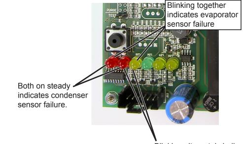
Blinking alternately indicates ice level sensor failure.
